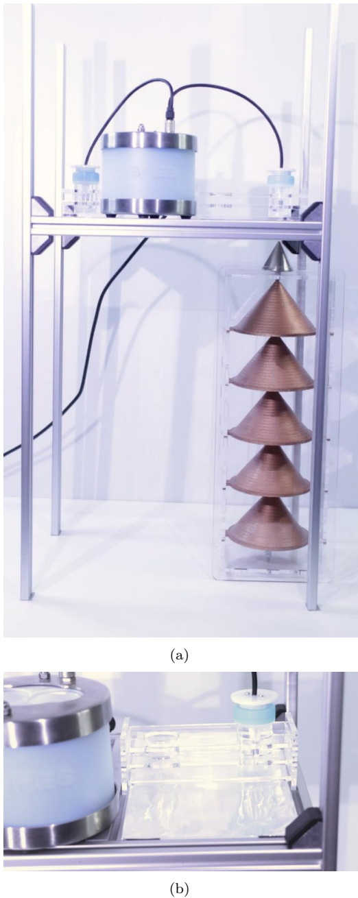
Fig. 11. (a) Experimental setup for differential exposure by 'Contur'; (b) Aluminium foil below the experimental container.
